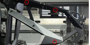
6. Install 6 of the factory clip nuts onto the locations shown below on our door panel. Make sure the orientation is correct in order for the bolts to seat properly.
