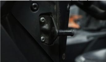
**16. Adust the paddle position** by sliding the position of the bottom paddle bracket bolt forward or back until the paddle is flush with the door in the rested position.
