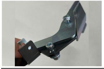
12. Install the supplied Spring by sliding it onto the bracket from the top and into the hole on the bracket. Then slide the other end of the spring onto the paddle and into the hole.
