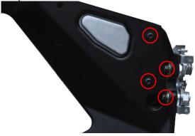
4. Drill out the 6 holes marked below using the supplied 23/64" drill bit. Install the supplied 6mm Rivet Nuts using a Rivet Nut Setter or you can use a bolt and a nut as shown in the video below.
