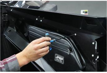
**9. Secure the rest of the door panel** reusing (6) of the factory Torx T40 bolts.
