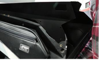
**8. Secure the top of the door panel** with (6) of the supplied M6 x 20 Button Head Screws and your 4mm Hex Key.
