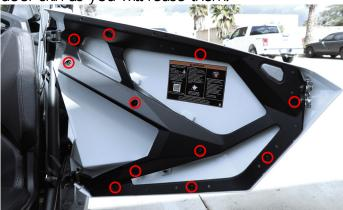
**3. Remove the factory paddle and latch** by removing the (2) Torx T30 bolts and the (2) 8mm bolts. You will reuse the factory latch, but not the paddle.
