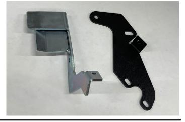
11. Place the supplied paddle on top of the paddle bracket and line up the top hole. Secure the paddle to the bracket with the supplied M6 socket head cap screws, #12 washers, and locknuts using your 5mm Hex Key and 10mm socket or wrench. The slotted hole in the middle of the paddle bracket will serve as a stopping point for your paddle. Make sure you install the washer on the nut side for the paddle to work properly. This will be adjusted in a later step.
