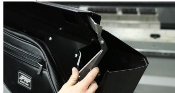
**14. Install the factory door latch** to the paddle and the door using the factory 8mm bolts.
