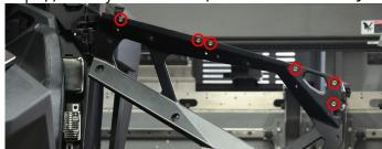
**5. Install the factory clip nuts** onto the supplied aluminum cutouts as shown below. These are needed to install PRP door bags. Save these for later use if you plan to install door bags at a later time. There are 3 on each door. Secure these pieces to the door frame with 3 of the factory Torx T40 bolts in the locations below.
