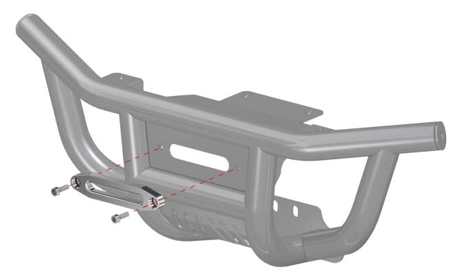
depending on Winch size, Fairlead may be smaller and require installation of provided Fairlead Adapter
