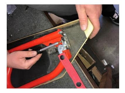
**Step 5:** Remount the stock door latches onto the Dirt Specialties door latch bracket in the center position using the stock bolts and washers. The latch mounts on the INSIDE of the door frame bracket. Replace the stock door latch strap if loose or torn.
