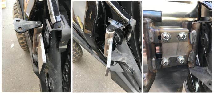
**Step 13:** Now install the rear doors onto the rear door hinge plates using the 4 supplied 8mm bolts and flat washers. Install the bolts from the inside of the car into the 4 slots in the center neutral position. Close the door and tighten semi tight.
