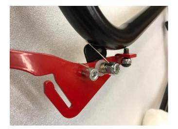
**Step 6:** Check the stock lower hinge pin for any burrs and file down before door installation. (Repeat on upper hinge if needed) Mount new supplied nylon washer onto the stock lower hinge pin. Place a small amount of lithium grease or other suitable lubricant onto the lower hinge pin.
