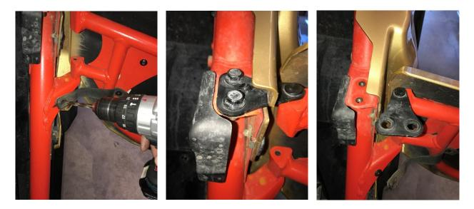
**Step 4:** Once on the work bench, remove the plastic latch covers. Now remove the original door latch from the stock doors and clean and oil the mechanism lightly if necessary for smooth action. Retain the bolts and washers.
